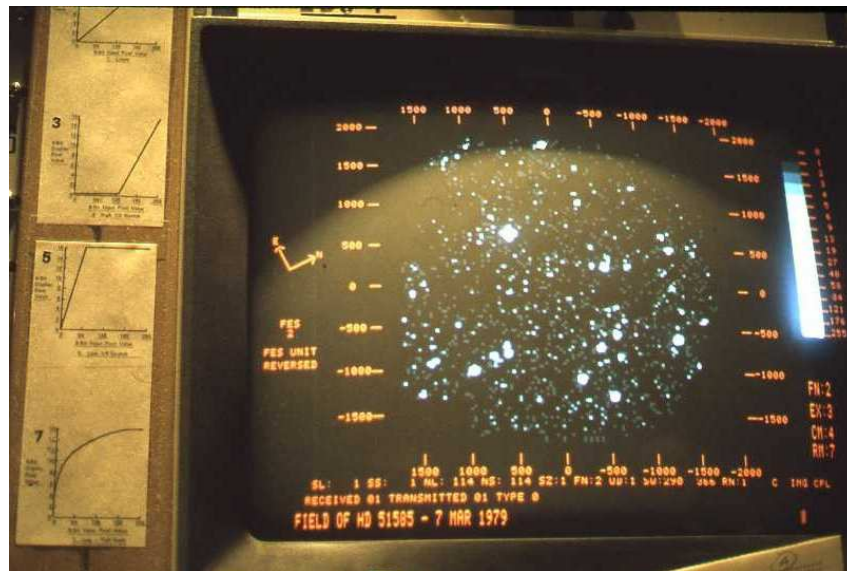
Fig. 83: Field of identification of a target (here HD51585) on the IUE Experimental Display System (EDS). Such fields had to be matched with the finding charts brought along by the V/As. PSS and ESO plates were used as backups. The faintest pixels might be background noise.
